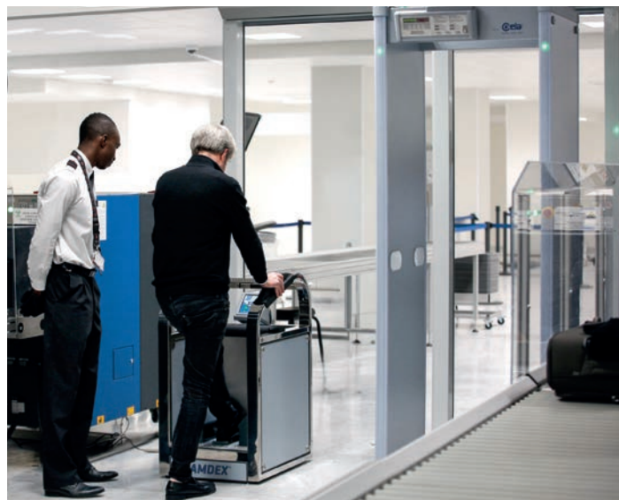
Passenger Screening by Walk-Through Metal Detector ( WTMD ), Shoe Scanner ( SAMDEX ) and passenger body control through PAT-DOWN
