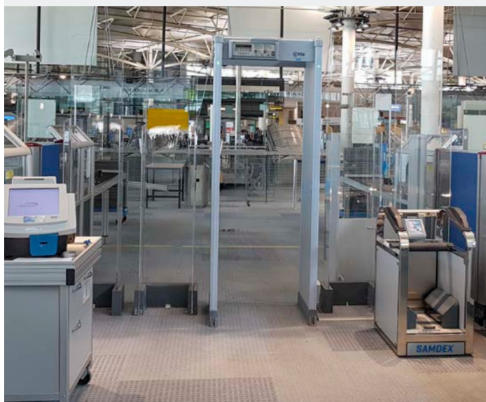
Passenger Screening by passenger body control through Security Scanner ( JANUS ) and Shoe Scanner ( SAMDEX )
