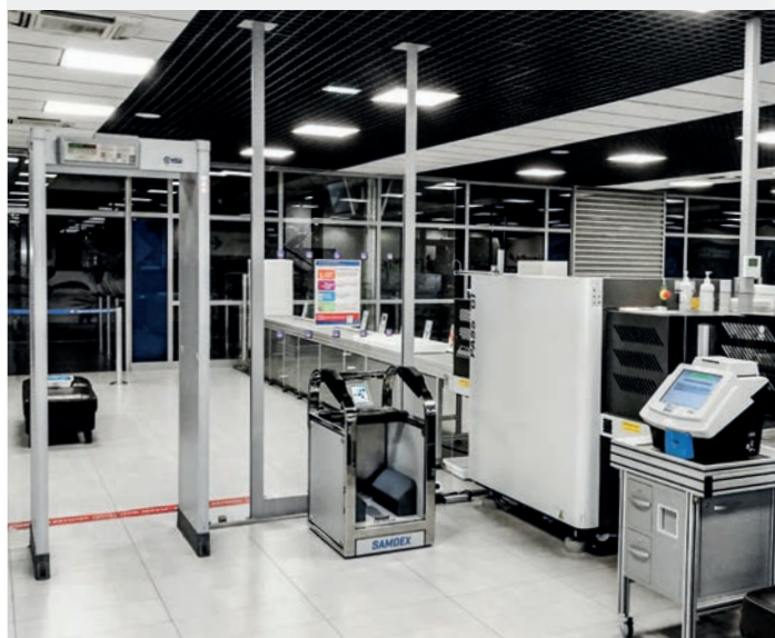
Passenger Screening by Walk-Through Metal Detector ( WTMD ), Shoe Scanner ( SAMDEX ) and passenger body control through PAT-DOWN
