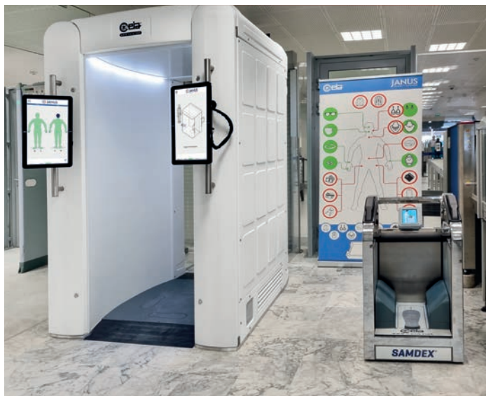
Passenger Screening by passenger body control through Security Scanner ( JANUS ) and Shoe Scanner ( SAMDEX )
