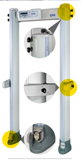
HEAVY DUTY CONFIGURATIONS are suitable for applications where the equipment is subject to frequent relocations. These models are characterized by cables with metal, military grade, connectors for quick plugging/unplugging and a rapid installation – all parts can be assembled without tools.
