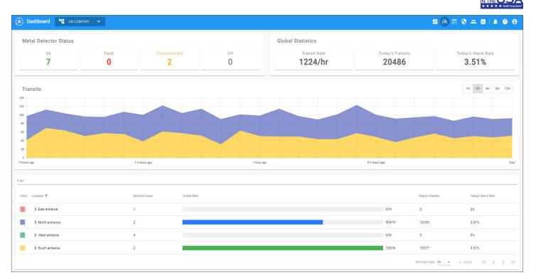
NetID Anywhere PREMIUM is a network management system for CEIA WTMDs and OPENGATE provided as a SaaS (Software as a Service). OPENGATE and the metal detectors communicate to the CEIA server via an LTE connection that operates on low power and does not effect the battery life. Security is provided by end-to-end encryption. There are no capital costs associated with the system and no installation of software is required.
