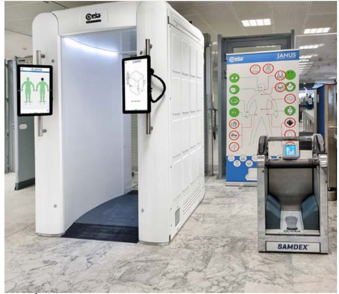
Passenger Screening by passenger body control through Security Scanner ( JANUS ) and Shoe Scanner ( SAMDEX )
