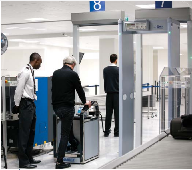
Passenger Screening by Walk-Through Metal Detector ( WTMD ), Shoe Scanner ( SAMDEX ) and passenger body control through PAT-DOWN
