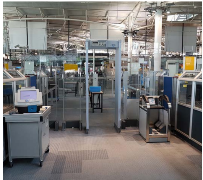
Passenger Screening by Walk-Through Metal Detector ( WTMD ), Shoe Scanner ( SAMDEX ) and passenger body control through Explosive Trace Detector ( ETD )
