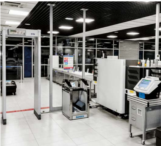
Passenger Screening by Walk-Through Metal Detector ( WTMD ), Shoe Scanner ( SAMDEX ) and passenger body control through Explosive Trace Detector ( ETD )
