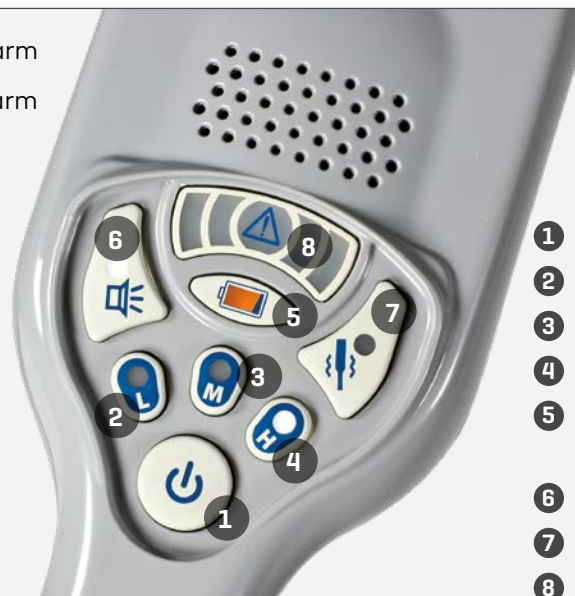
Optical indication proportional to the radioactive substance signal strength.
