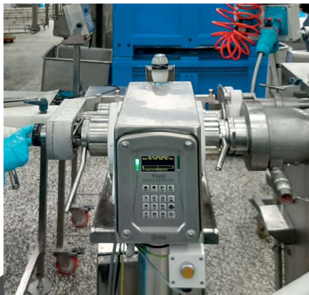
THS/PLH21 MODEL WITH INTEGRATED TWISTING EXTENSION KIT
